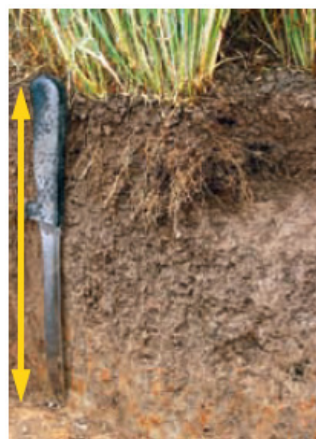
Figure 4: Soil density and potential for rooting depth may be determined in the soil profile by number and distribution of root canals, cracks, and earthworm tunnels FAO (2008) VISA – Visual Soil Assessment Guide. Verfügbar unter: http://www.fao.org/3/i0007e
